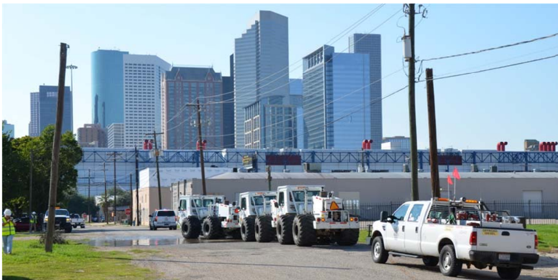
Figure 5. Acquiring seismic data in downtown Houston for EAS professional MS research, sponsored by Dawson Geophysical with field crew and vibroseis trucks.
