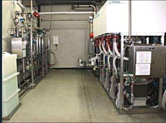
1 MW PEM electrolyzer: 272,000 cm 2 11,000x test cell
